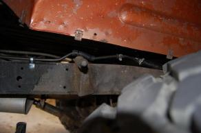
The Sniper has a built-in fuel pressure regulator, which requires a return line to the tank. For this run I used the same combination of fuel lines and added a tee fitting to the tank's filler neck vent line.
