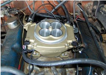
The kit comes with several different brackets to connect most throttle and kickdown linkages to the unit. Unfortunately, at the time of this installation, Holley did not offer a bracket to connect the original kickdown rod for the C4 automatic. Instead, I purchased a kickdown cable from <a href="BC Broncos">BC Broncos</a> and modified one of the brackets that was included in the Sniper kit to connect it to the throttle body.
