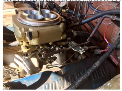
The system comes with a coolant temp sensor that I installed in place of the existing aftermarket sending unit I had in the intake manifold. Also included with the kit is an O<sub>2</sub> sensor and a clamp-on threaded bung that's designed to allow you to be able to install the sensor without welding-in a permanent fitting. The clamps that
